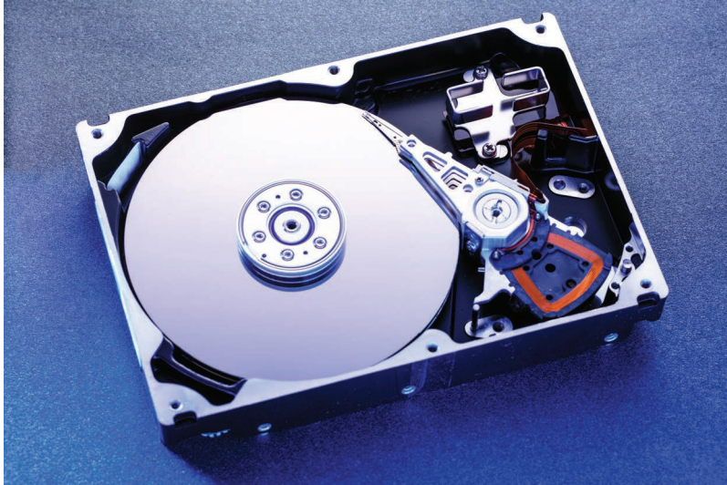
Figure 11.2 A 3.5-inch HDD with cover removed.
