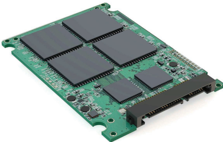
Figure 11.3 A 3.5-inch SSD circuit board.
